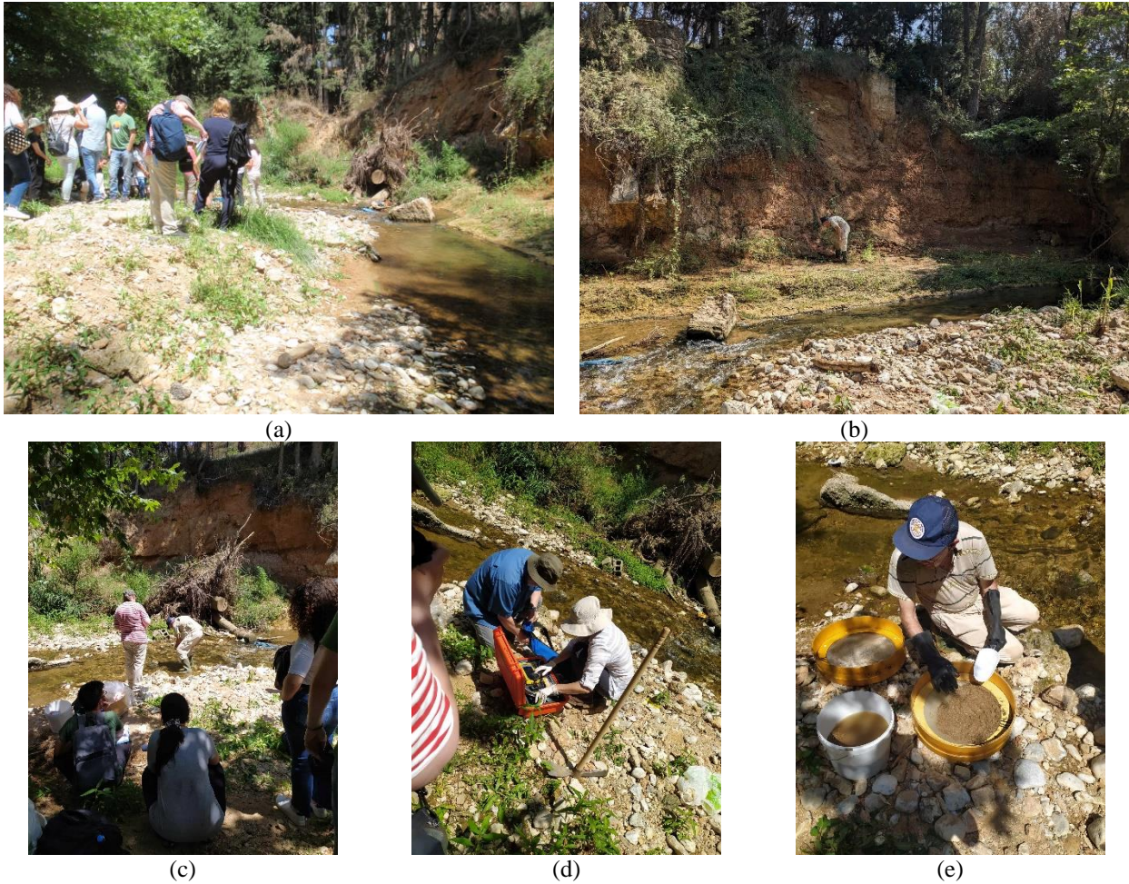
Figure 8. (a) Stream water, Stream sediment and Overbank sediment site; (b) Overbank sediment section; (c) Stream water sampling; (d) stream water measurements, and (e) Sieving of active stream sediment. Demonstration of field sampling methods by Hatakka Tarja and Alecos Demetriades, and stream water measurements by Konstantina Tsoulou.
