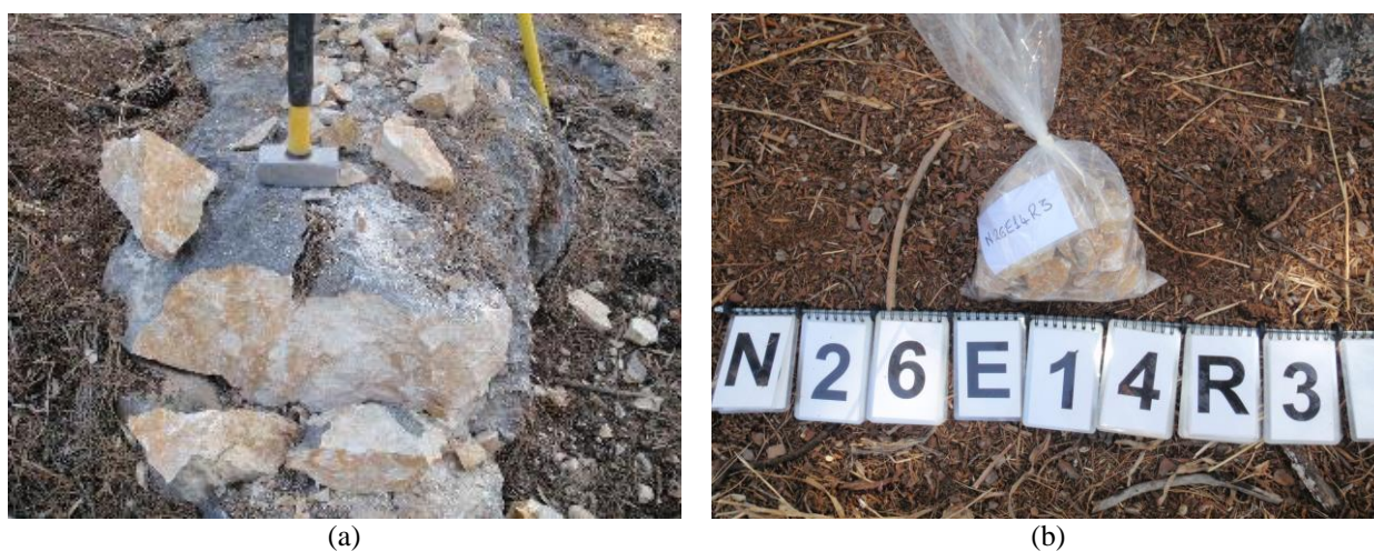
Figure 5. Demonstration of rock sampling by Alecos Demetriades: (a) Breaking up of outcrop, and (b) bagged rock sample with its Global Terrestrial Network (GTN) sample site number.
