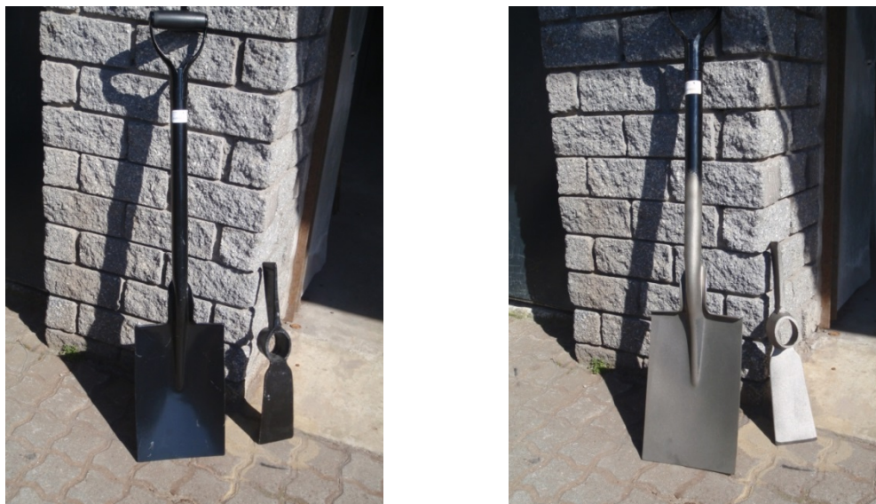
Figure 30. (left) Painted spade and mattock cutter, and (right) Sandblasted spade and mattock cutter; the paint on part of the handle was left for demonstration purposes.
