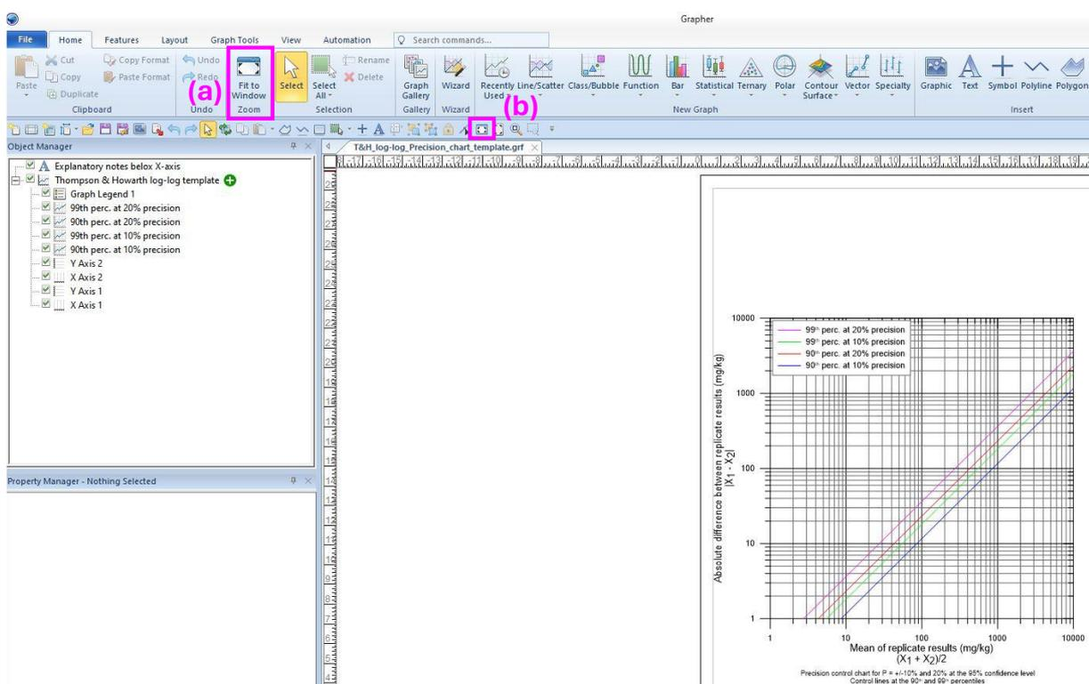
Figure 6. The opened template is enlarged by using the command 'Fit to Window Zoom' with a left mouse click; there are two options, either (a) or (b), that can be used.
