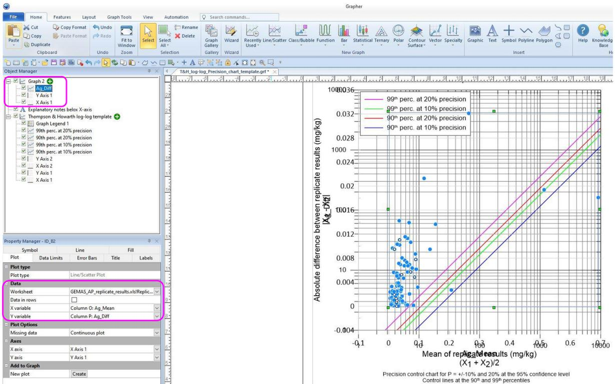
Figure 12. The graph of Mean versus Absolute Difference of the Ag replicate results is displayed. It is noted that on top of the template's X and Y axes names, Ag\_Mean and Ag\_Diff are superimposed; this also applies to Figures 13 and 14.
