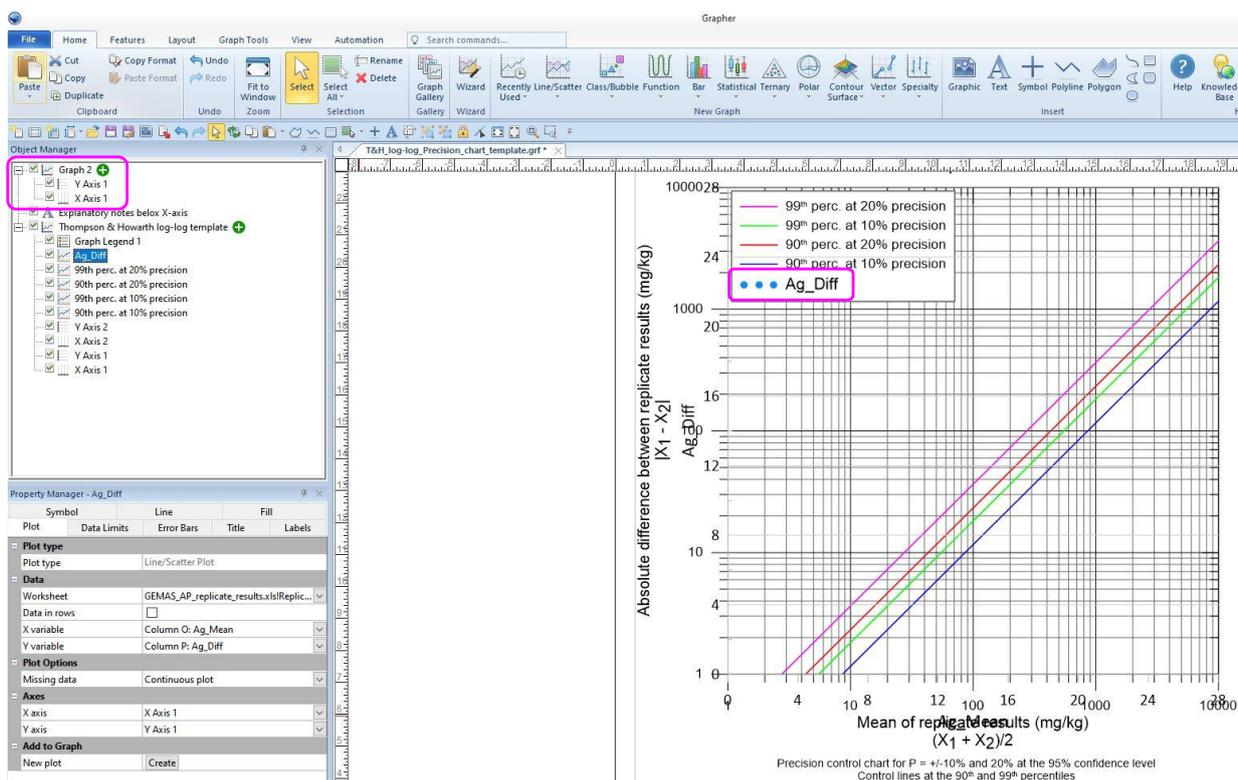
Figure 14. After moving the Ag replicate pairs (Ag\_Diff) to the main Thompson and Howarth log-log chart, and selecting the plot axes (Fig. 11), the blue dots of the Ag replicate pairs disappear from the chart. Since Graph 2 is no longer needed, delete it by marking it and then pressing the command 'Delete'.
