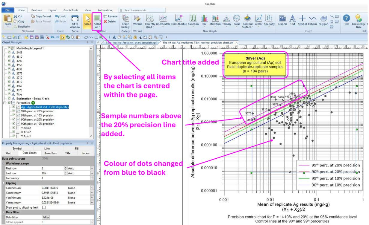
Figure 18. Annotated figure showing all the changes made.
