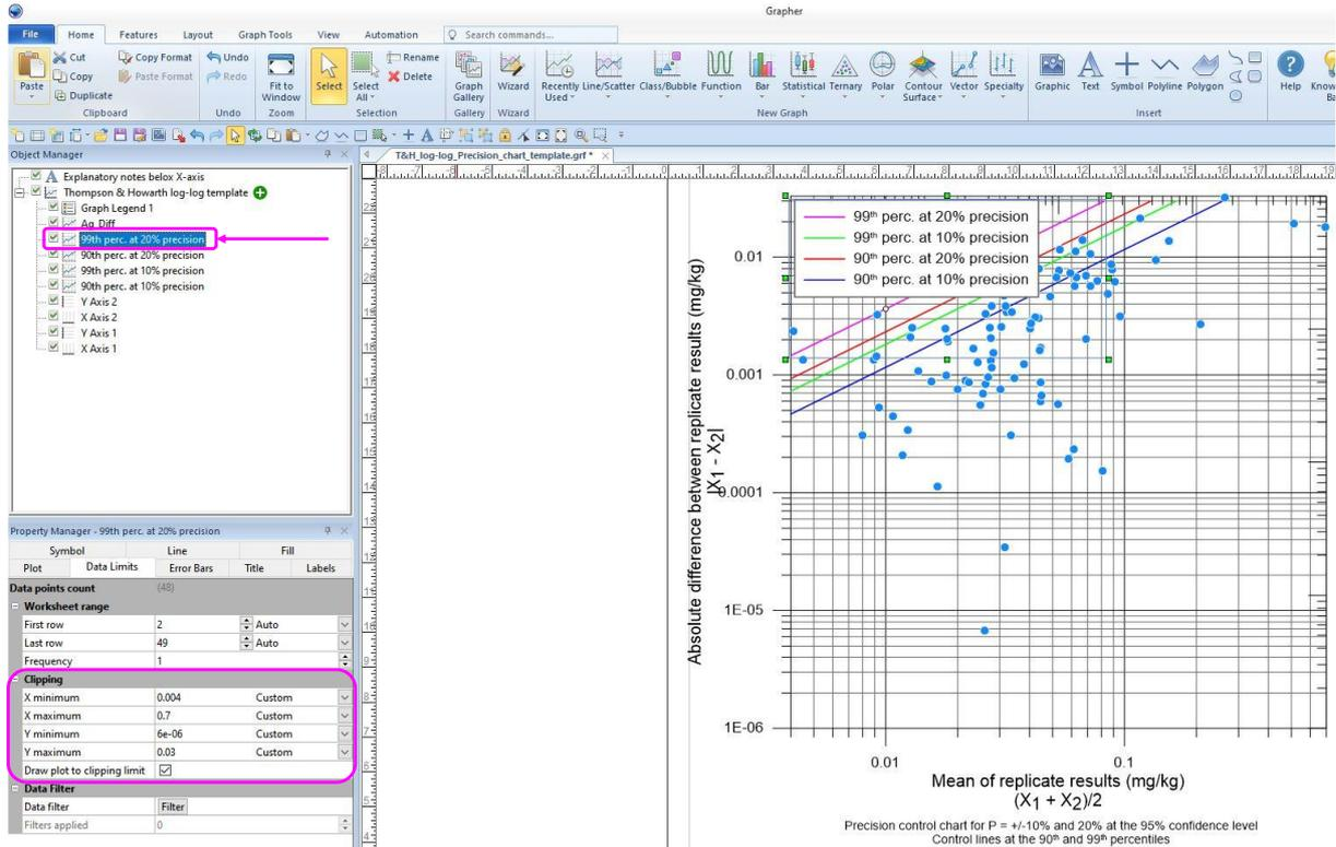
Figure 16. After changing the minimum and maximum values of the four control lines, they appear within the plotting area of the Thompson and Howarth  $\log_{10}$ - $\log_{10}$  chart.
