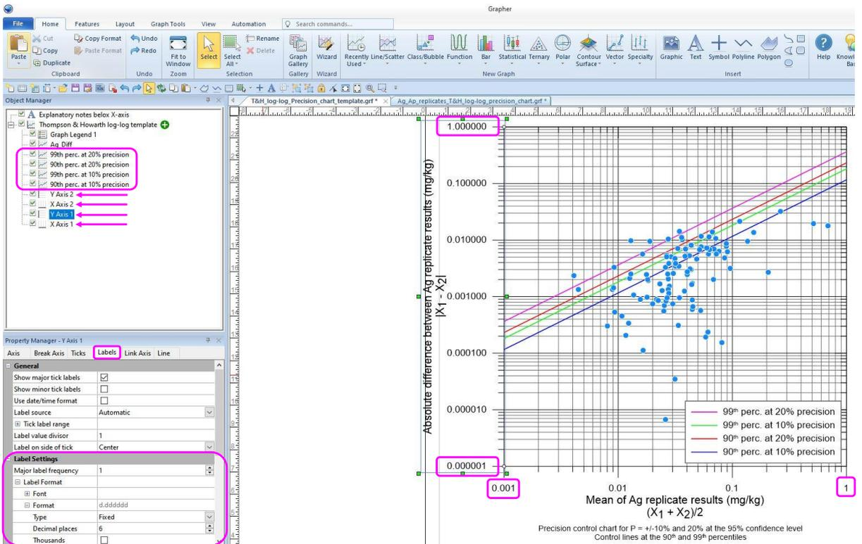
Figure 17. Final touches to the chart: (a) Minimum and maximum limits of  $X_1-X_2$  and  $Y_1-Y_2$  axes changed; (b) limits of the precision lines changed, and (c) the decimal places of the Y-axis changed by selecting 'Labels' in the Property Manager, and selecting 'Type' and assigning 'Fixed' and then 'Decimal places' to 6.
