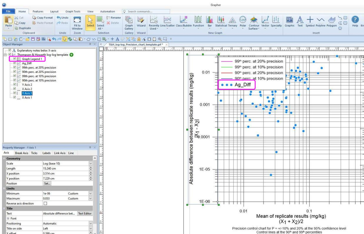
Figure 15. After changing the minimum and maximum values of the X and Y axes, the Ag replicate pairs appear within the plotting space of the Thompson and Howarth log-log chart. The entry '...Ag\_Diff' is removed from the legend box.
