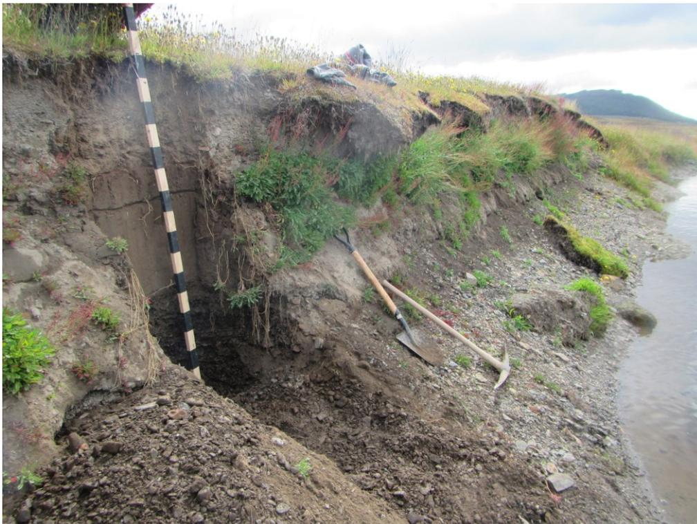
Figure A4.14. Field site JP-765. The exposed overbank sediment bank on Ransmunssen River is adjacent to its junction with route Y-895. The bank was cleared to expose the overbank sediment sequence, and a pit dug down to the bedload deposit. Photograph by Juan Lacassie (SNGM).
