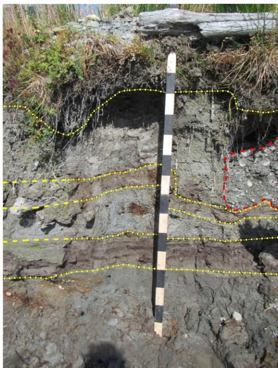
Surface layer, apart from the vegetation, consists of polymictic clasts with medium to coarse sand-sized sediments and abundant organic matter; the tree trunk and clasts were possibly deposited during the last flood.
